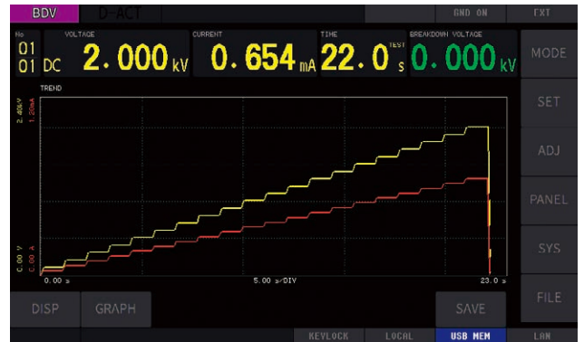
Example of stepped voltage rise testing
