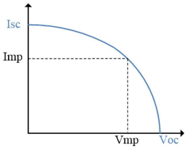
to set the I-V characteristics of the PV cell ( $V_{oc}$ ,  $I_{sc}$ ,  $V_{mp}$ ,  $I_{mp}$ ). Use the inverter to test its static MPPT performance.
