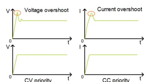
moment the output is turned on, effectively avoids the current or voltage overshoot resulted from capacitive or inductive load.
