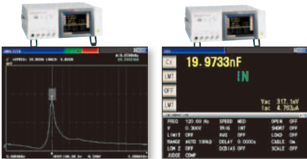
Frequency sweep measurement Z peak comparator screen
