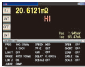
LCR mode Rs display screen (100 kHz measurement)
