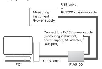
\* A GPIB interface by National Instruments, Keysight, or Contec (32 bit only) is required.
