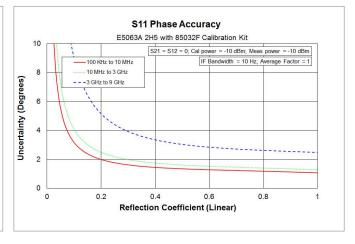
1. The performance from 50 kHz to 100 kHz is the same with one from 100 kHz to 10 MHz as typical.
