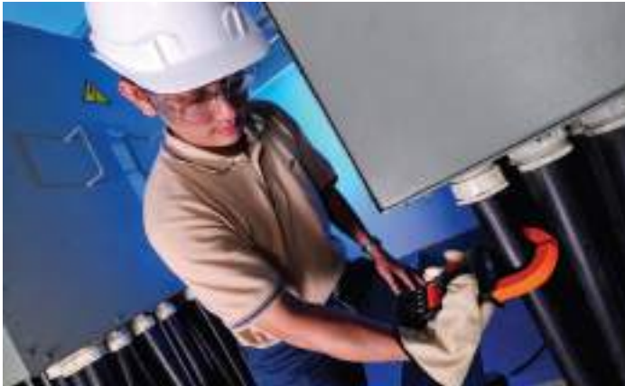
Figure 2. Large jaw clamp opening of 52mm / 2 inches
