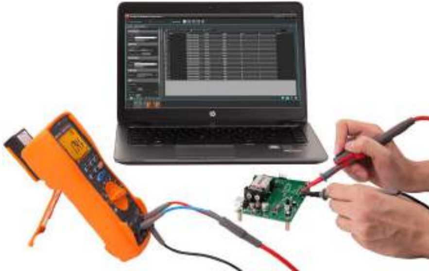
Figure 6. Data logging experience with Keysight Meter Logger software
