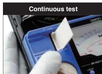
Lift and lock the MEASURE key to apply a continuous stream of voltage
