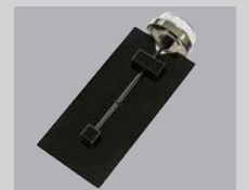
Black panel thermometer (for calibrating BPT sensor)
