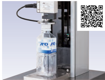
Plastic bottle compressive strength test
