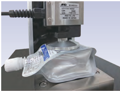
Packing container compressive strength test
