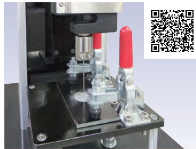
Food packaging puncture test
